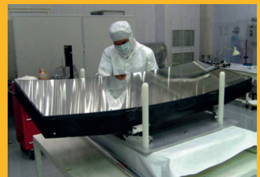
Final verification of one of the Gaia primary mirrors
